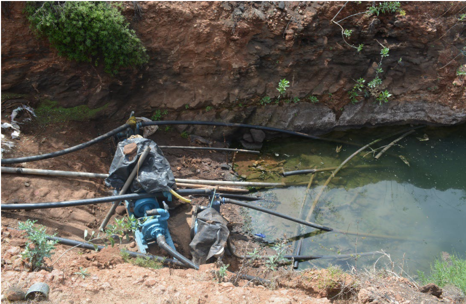
Figure 2: Diesel pumping abstracting water from the sand river
